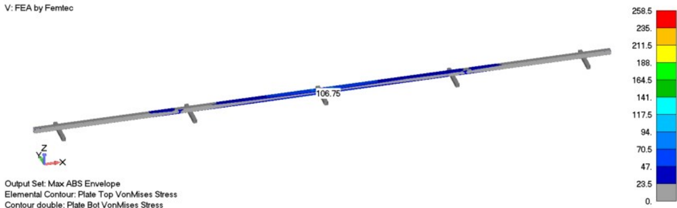
Figure 24: Von Mises stresses main steel beams
